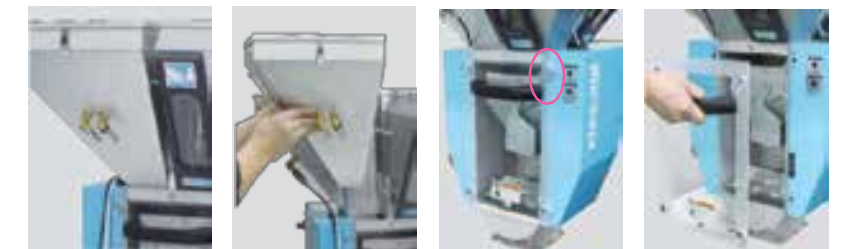
Material Hopper properly mounted Dismounting material hopper. Door Closed Door open
