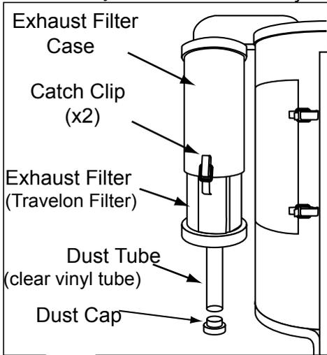
Note: The surface temperature of the exhaust filter will run up to 130°C when operating. Do not come into contact with filter.
